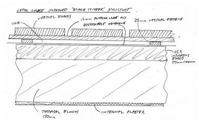
The inner layer of boards is replaced with 12mm ply on 25mm battens. Behind that is a breather membrane (Tyvek, Nilvent, etc) and a layer of solid insulation board (Celotex GA4000 or similar).
